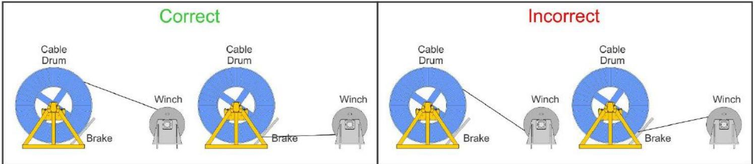
Wire rope should be attached at the correct location on a flat or smooth-faced drum, so that the rope will spool evenly, with the turns lying snugly against each other in even layers. If wire rope is wound on a smooth-face drum in the wrong direction, the turns in the first layer of rope will tend to spread apart on the drum. This results in the second layer of rope wedging between the open coils, crushing and flattening the rope as successive layers are spooled.
