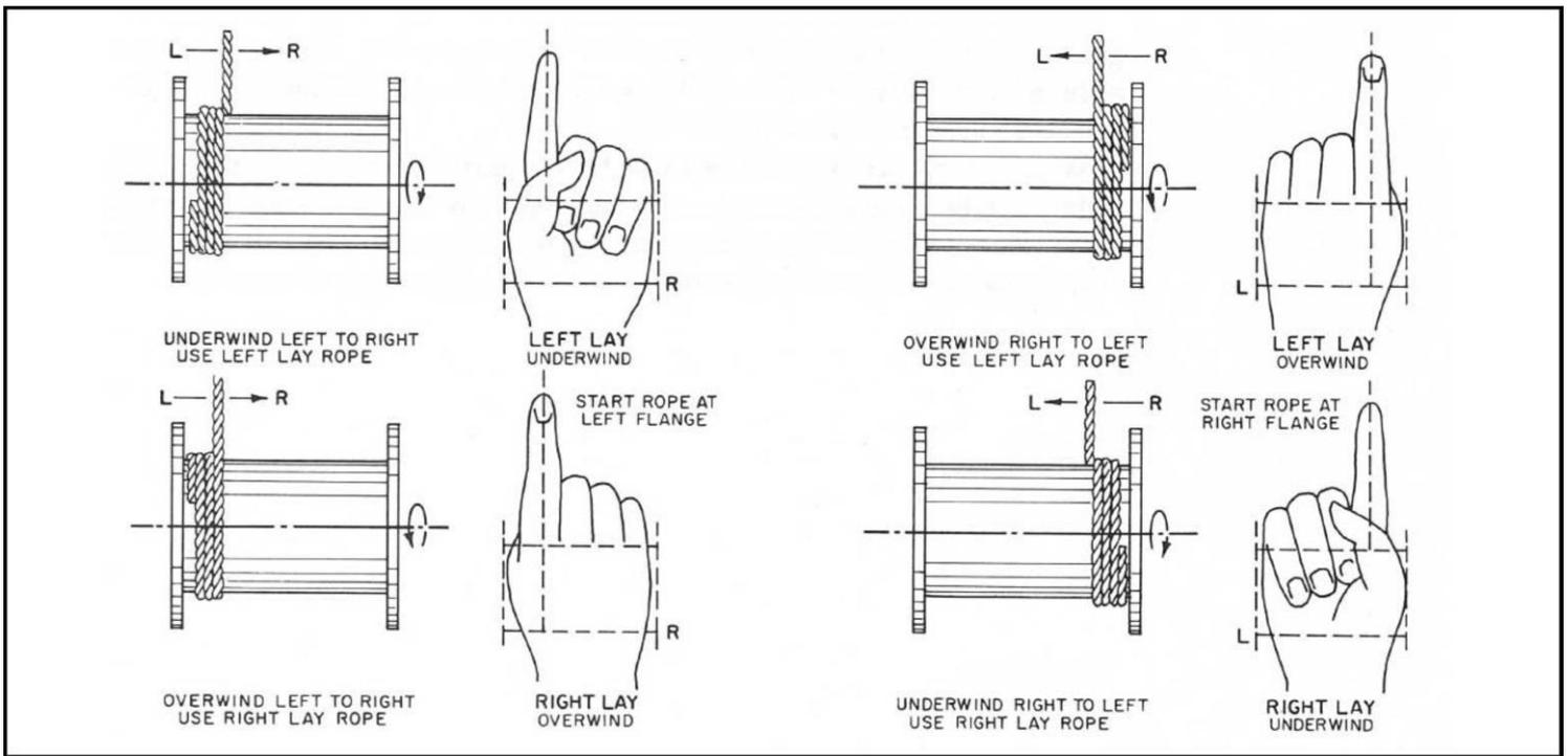
A simple method of determining how a wire rope should be started on a drum is shown above. The observer stands behind the drum, with the rope coming towards him. Using the right hand for right-lay wire rope, and the left hand for left lay wire rope, the clenched fist denotes the drum, the extended index finger the oncoming rope.
