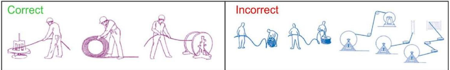
**Uncoiling a Wire Rope** - There is only one correct way to uncoil wire rope. Again, it is a two-person job, whereby the first person holds the end of the rope, while the second person rolls the coil along the floor, backing away. The rope must be allowed to uncoil naturally with the lay, without spiralling or twisting. Always uncoil wire rope as shown below.
