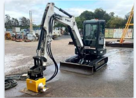
Quick-Hitch Capstan Winch Mounted on an Excavator
